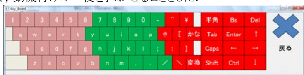
Fig. 3 Virtual keyboard on the PC-monitor Four colors are corresponding to colors of those four button switches shown in Fig. 1.
