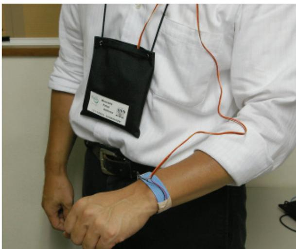
Fig. 3 The radio receiver and the vibrator
