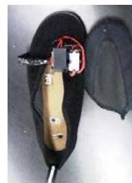
Fig. 1 device of shoe type stabilograph
