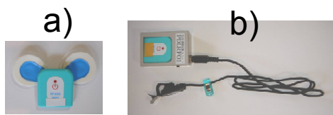
Fig. 1 Wireless sensors for measuring a) ECG signal and b) photo-plethysmographic signal
