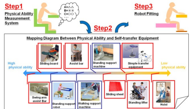
Fig. 2 Algorithm for selecting appropriate self-transfer equipment based on the physical ability of the user
