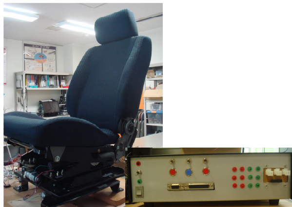
Fig.5 Electric power seat and the control system
