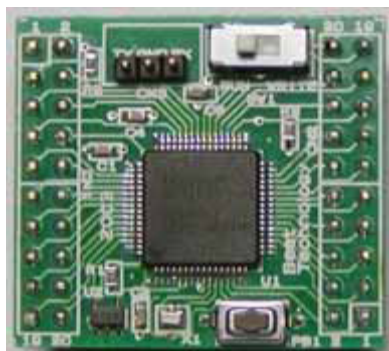
Fig.6 H8/3694 CPU Board
