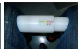
Fig.2 Knee-gap force measurement device
