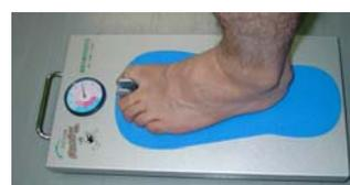
Fig.1 Toe-gap force measurement device
