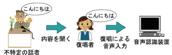
Fig. 1 An overview of the proposed speech recognition system collaborating with a re-speaker.
