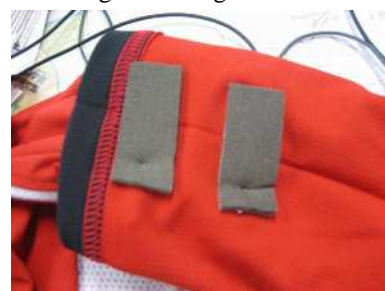
Fig. 4 Conductive Sponge Electrode
