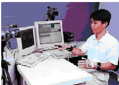
Fig.1 Sign language translation that uses camera and cyber glove by Hitachi, Ltd. (2001)
