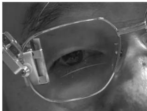
Fig. 2 Positioning of the sensor array relative to one of the subject's eyes by means of a 3-DOF sensor attachment secured to an eye-glass
