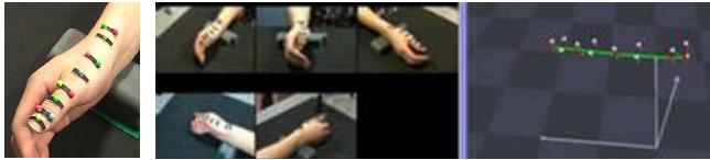
Fig. 6 Experimental situation to measure a fingertip motion
