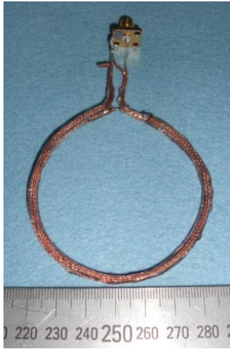
Fig.12 Measurement device of blood relative permeability using coaxial cable coil of 2 turns
