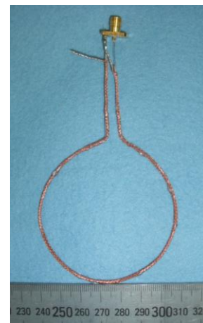
Fig.7 Measurement device of blood relative permeability using coaxial cable
