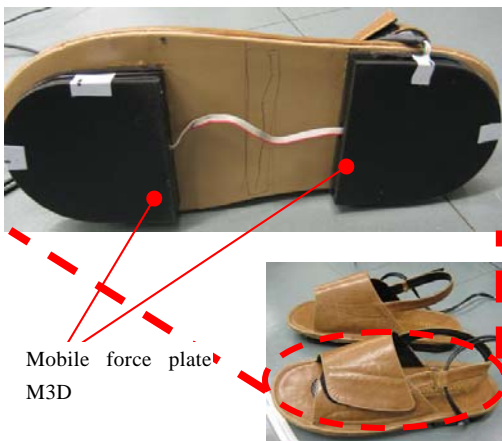
Fig. 5 Wearable ground reaction force sensor system (2 mobile force plates M3D attached to a flexible foot wear ).
