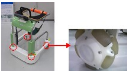
Fig.1 Omni-directional walker and its omni wheel
