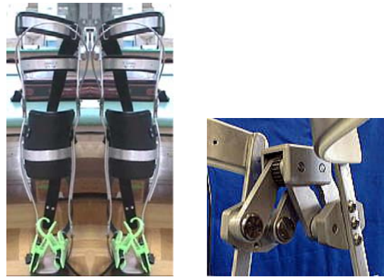
Fig.1 KAFO of hip joint with medial single link type & Link type hip joint.
