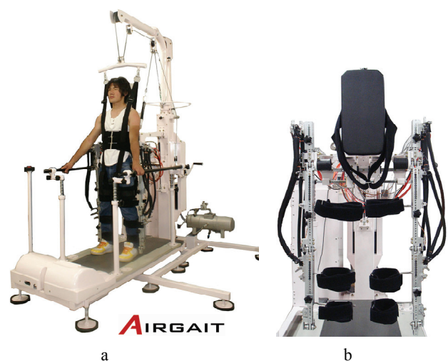
Fig. 2 Body weight support gait training system “Airgait”
