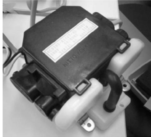
Fig. 3 Diaphragm pump
