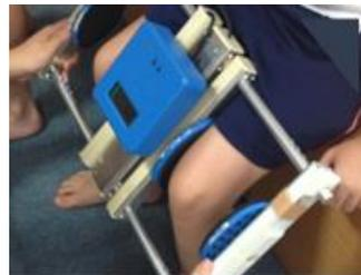
Fig.4 The knee-gap force measurement device
