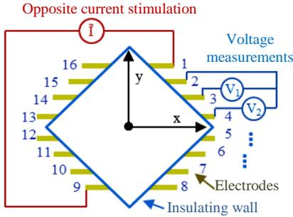
Fig 3 One section of microchannel and measurement strategy
