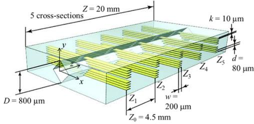
Fig 2 Dimension of the microchannel
