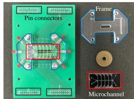
Fig 1 Photo of microchannel and connections
