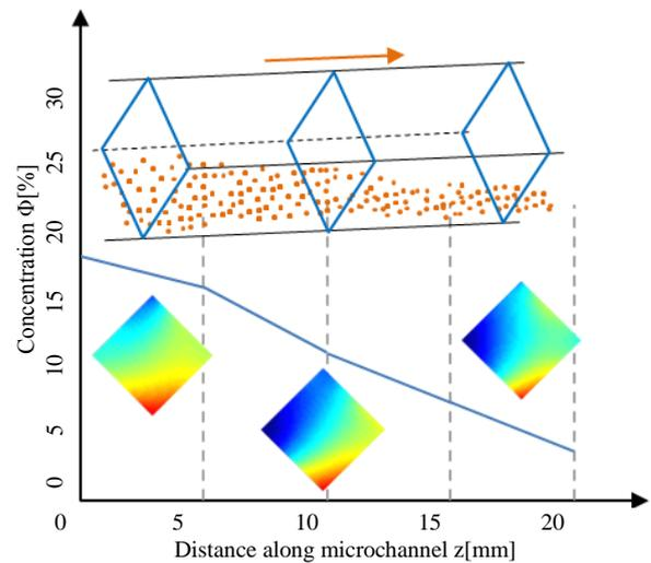
Fig. 5 Application of cell visualisation in the  $\mu$ EIT system
